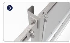
The Powerway vertical mounting system enables new approaches for the utilization of solar energy especially in agricultural areas. The solid steel construction consists of mullions and cross beams. Two mullions and three crossbeams hold vertically bifacial modules.
