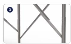
The incorporation of a diagonal brace design significantly strengthens the structural framework, enabling it to withstand higher loads and providing greater stability and durability under various conditions.
